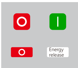
Circuit breaker is disconnected and no energy storage
